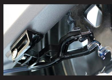
The new Multiform Dispenser Mounting Bracket utilises adhesive pads for a quick and easy installation. The **Scorpion** Dual Injector can be fitted to a variety of swingarm types and in different orientations allowing for compatibility with a greater number of different makes and models. The bracket can be easily adjusted, to easily accommodate chain adjustments
